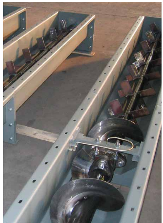
Aisi 304 grade steel screw diameter 1600 for transporting sugar.
