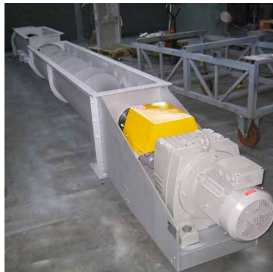
Integrated mobile plant complete with hopper and screw conveyor.
